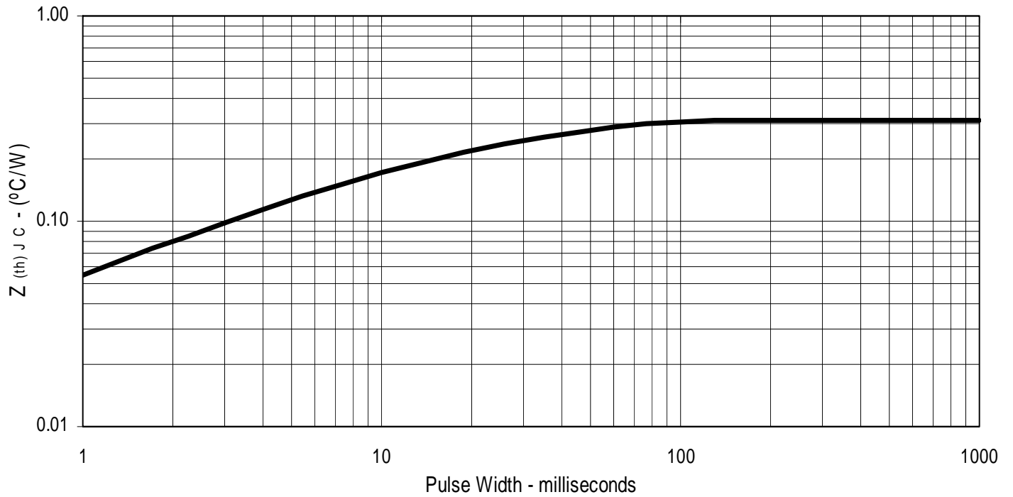
Fig. 13. Maximum Transient Thermal Impedance
